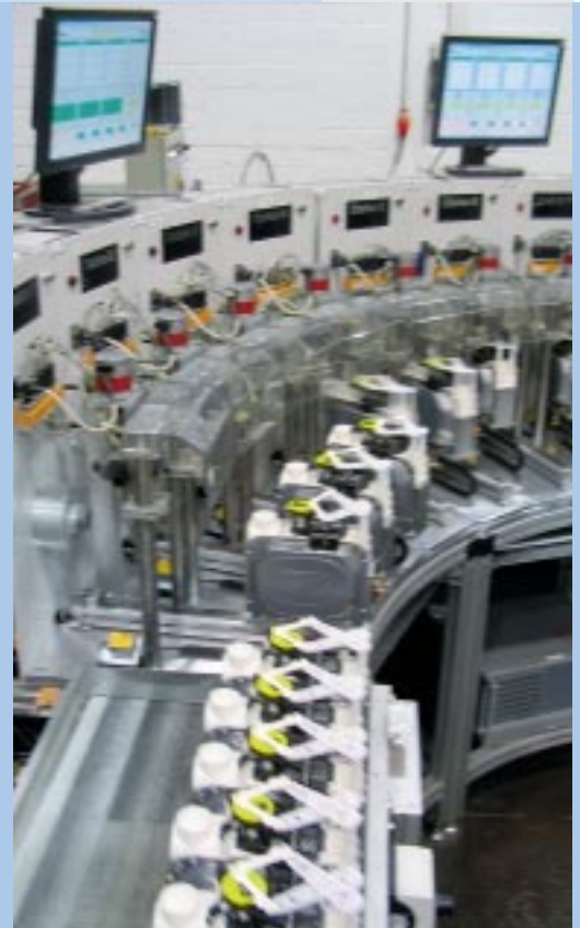
Fig. 3: Automatic pre-calibration of measuring units
