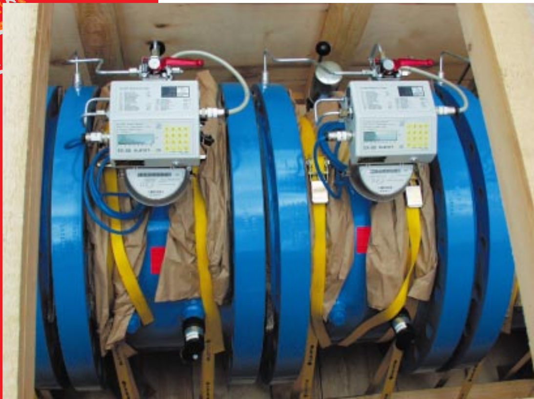
Elster high-pressure turbine meters ready for the long trip
