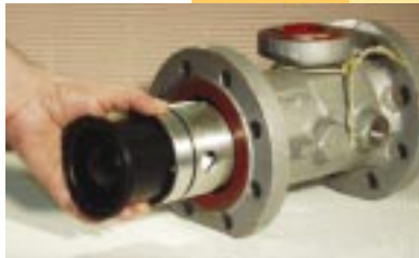
Fig.1: Exchanging a measuring cartridge at Elster
