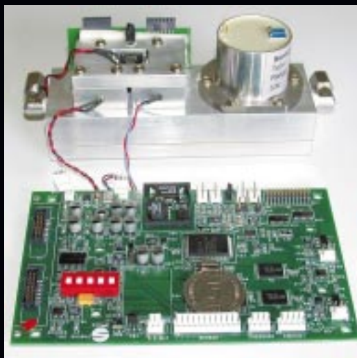
Fig. 4: Sensor block and primary electronics of the gas-lab Q1
