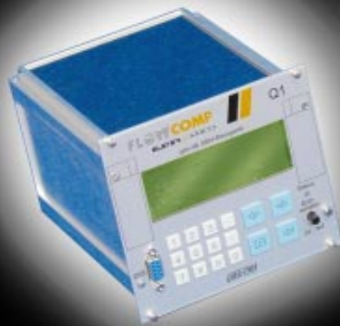
Fig.1: Measuring the gas quality using a correlation procedure with spectroscopic and thermal values
