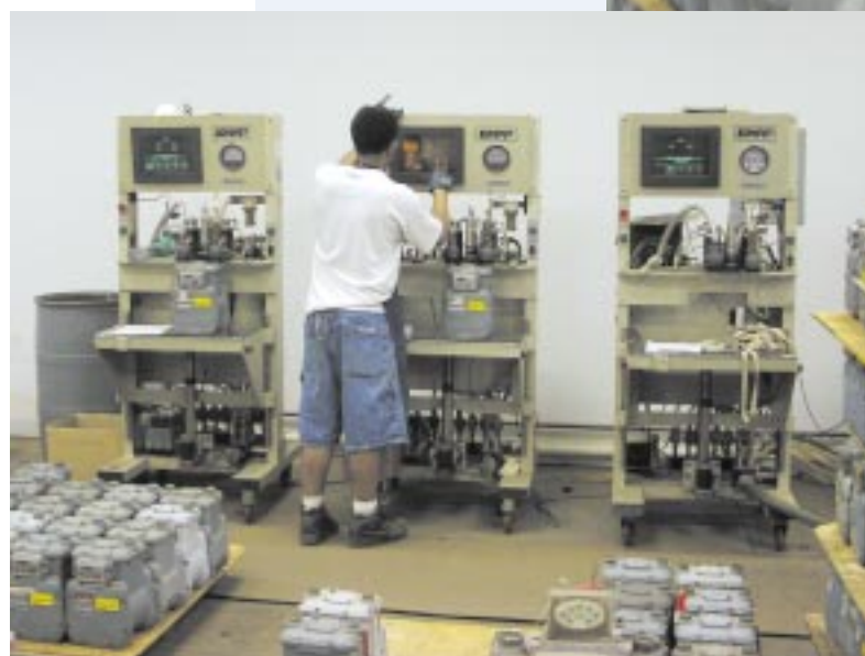
Proving meters using the sonic nozzle prover
