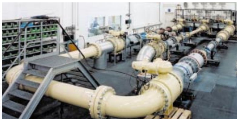
Fig. 1: High pressure test rig pigsar, capacity up to 6500 m 3 /h, test medium natural gas, pressure up to 50 bar
