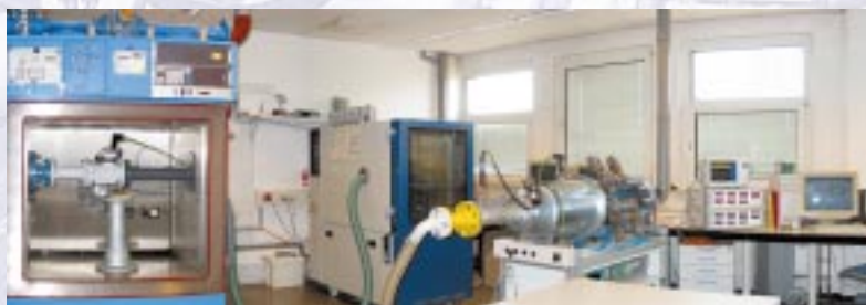
Fig. 2: ELSTER temperature lab, -50 °C to +80 °C, capacity up to 100 m 3 /h
