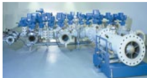
Fig. 3: ELSTER test rig, capacity up to 12000 m 3 /h, test medium air
