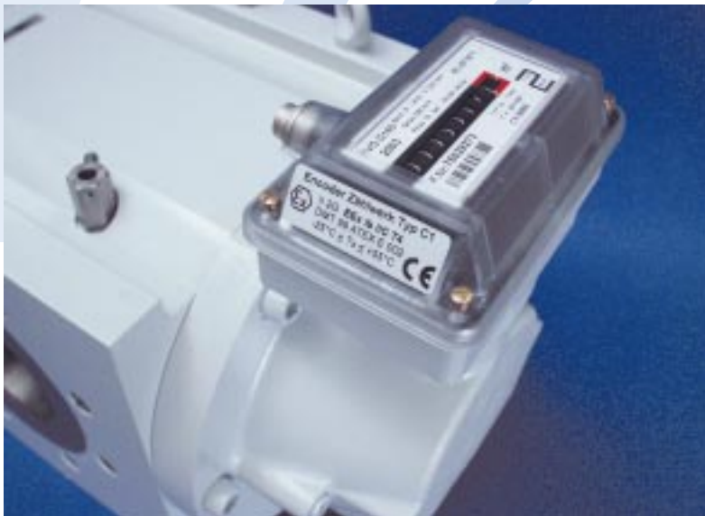
Fig 1: New Encoder index on an RVG
