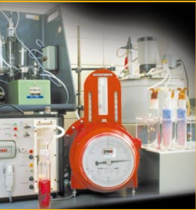
Laboratory gas meter, dry version (left) and wet version (right)
