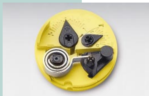
Fig. 2: Measuring unit of a BK-G4 with TC
