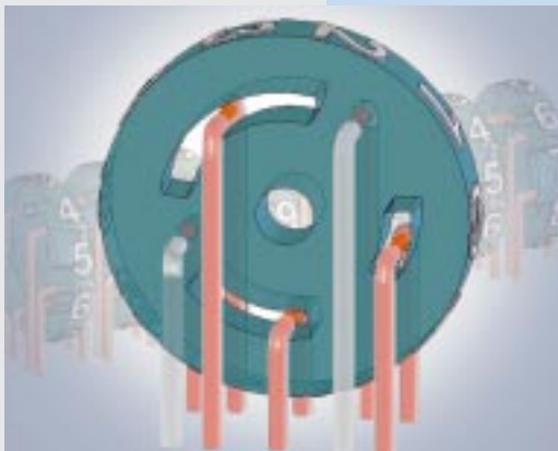
Optical detection principle of the ENCODER
