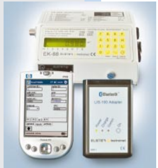
Fig. 3: Software module RM100 together with wireless interface also supports the older devices, e.g EK-88
