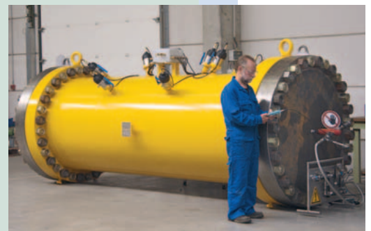
Fig. 3: Multi-path 48" Q.Sonic performs Factory Acceptance Test (FAT)
