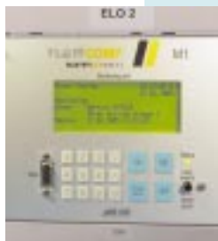
gas-net M1n message and monitoring unit
