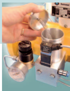
Fig. 3: Automatic oil pump
