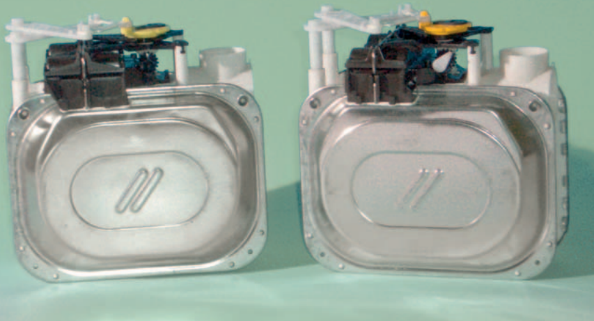
Fig. 1: Brothers, but not identical twins: the measuring units of the BK-G6 V2 (left) and the BK-G4 V2
