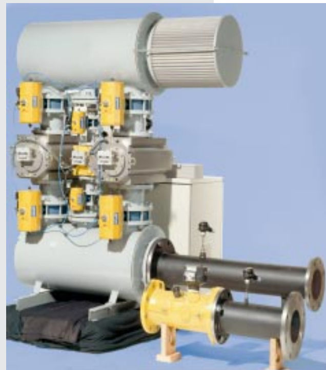
Fig. 2: Test bench ITF from Elster-Instromet with IRM DUO meters as master meters
