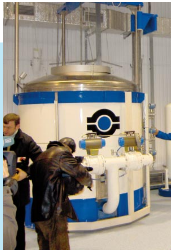
Fig. 2: Bell prover and weighing tank Primary Standards
