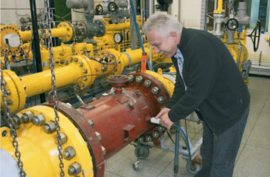
Ulrich Müller checks the pulse transfer of a measuring cartridge under test
