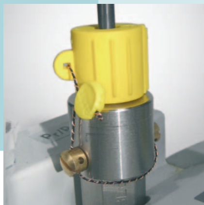
Fig. 3: Adapter for old thermowells EBL50/67
