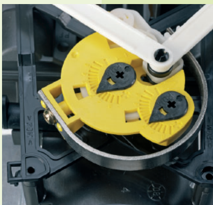
Fig. 2: Bimetallic element on measuring unit V6 A bimetallic element fitted in the crank mechanism changes the crank radius as the result of a deflection if a temperature change occurs in the measured gas. This changes the diaphragm stroke causing a change in the volume of the measuring chamber proportional to the absolute gas temperature.
