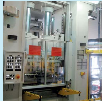
Deep drawing line with modern anti-friction coating technology
