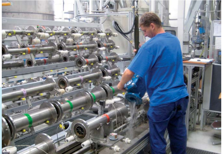
Computerised testing line for C&I water meters
