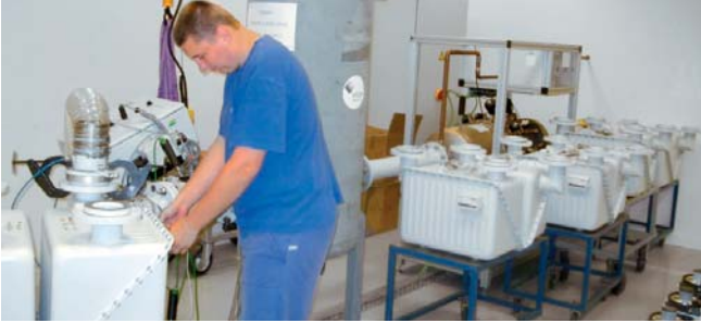
Modern sonic nozzle test rig for rotary and industrial diaphragm gas meters
