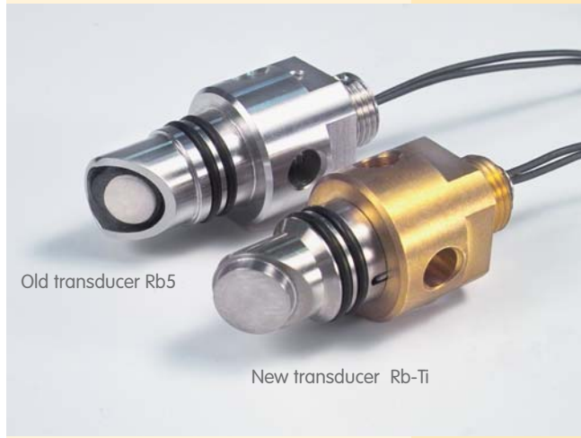
Two-part design: The wetted part is made of titanium, the connection block of brass.
