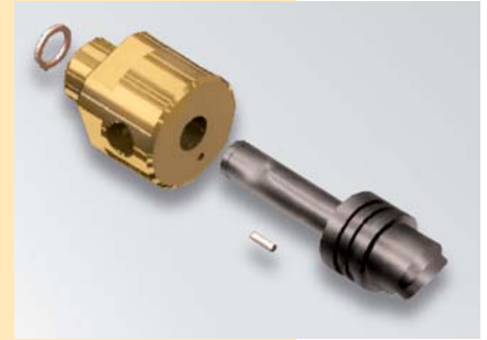
Two-part design: The wetted part is made of titanium, the connection block of brass.
