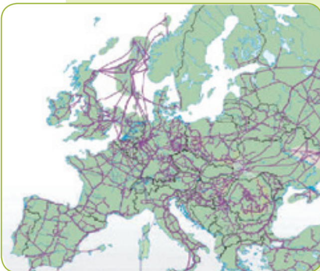
Gas pipeline network in Europe with an overall length of more than 200,000 kilometres
