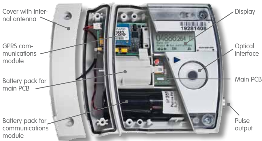
Fig. 3: The modularity of the electronic index
